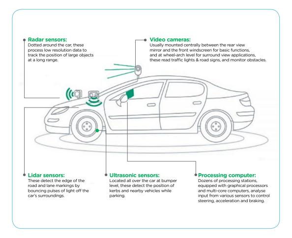
Figure 4 Some of the technologies that support automated driving<sup>7</sup>
