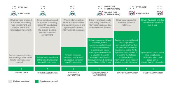
Figure 5 Levels of driving automation (based on the SAE International J3016 Standard)9
